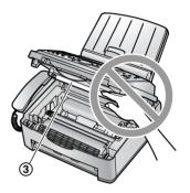
5 Clean the document feeder roller (①) with a cloth moistened with isopropyl rubbing alcohol, and let all parts dry thoroughly. Clean the upper glass (②) with a soft and dry cloth.
